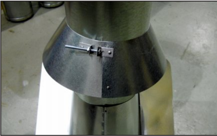
Figure 7.14 - Insert Bolt into Brackets
