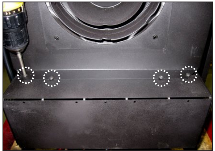
Figure 8.5 - Attach Blower with Four Screws
