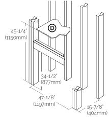
The fireplace enclosure must be a minimum 45-1/4" (1150mm) tall. Do not build into the fireplace enclosure.
