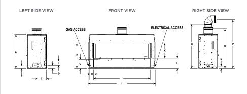
3: Framing depth will vary if you are installing the low profile power vent (PVLP-SLP) with minimum vent configuration. 12-1/2" is needed from the back of the appliance to the outside of the exterior wall. Refer to manual for details.
