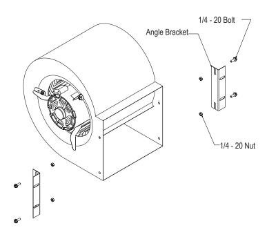
2. Attach blower to the left and right mounting brackets.
