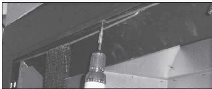
Figure 3.9 Removing the Screen Rods
