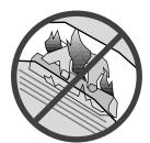
The viewing glass should be opened only for conducting service. Do not operate with cracked, broken, or removed glass.
